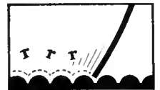
This is the action of the usual wire wound control after it has been in use for some time . . . like dragging a stick over a cobblesone pavement.
