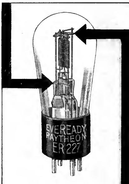
Showing the exclusive patented Eveready Raytheon 4-Pillar construction. Note the sturdy four-cornered glass stem through which the four heavy wire supports pass, and the rigid mica sheet at the top.
