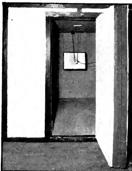
Fig. 2—Interior view of the sound-proof room in which loud speaker measurements are made.
